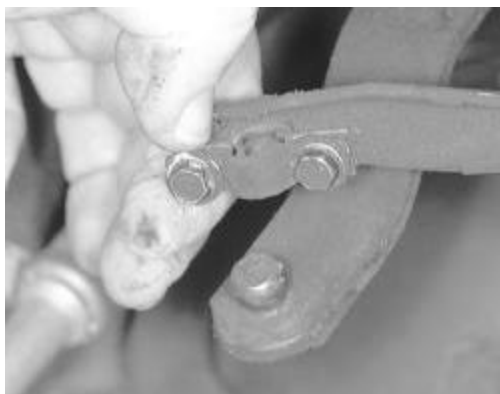
Fig. 1: You must disconnect the wiper linkage to allow clearance for removing the heater core coolant ho
