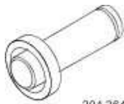
Pinion seal installer 204-264
