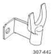
Halfshaft splitter 307-442
