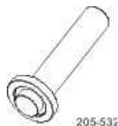
Halfshaft oil seal installer 205-532
