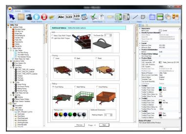
Putting together smart wizard like input screens eliminates confusion and incompatible designs allowing non-technical users ability to produce drawings, 3D models and bills of materials.
