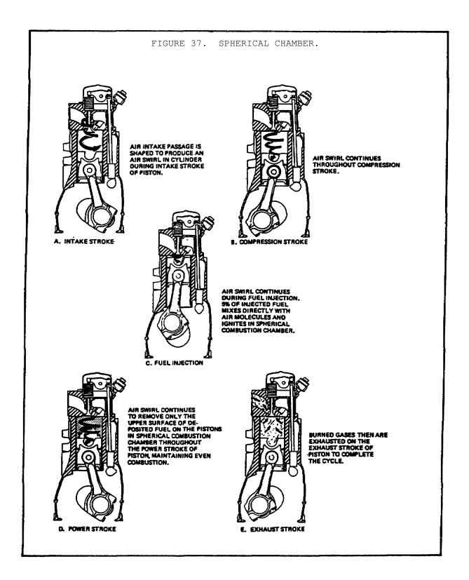
(1) As the air enters the combustion chamber, a swirl effect is introduced to it by the shape of the intake port (figure 37, view A).
