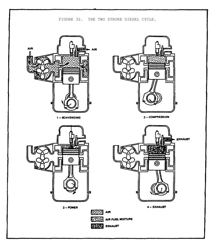
(2) Compression. As the piston moves toward top dead center, it covers the intake ports. The exhaust valve closes at this point sealing the upper cylinder. As the piston continues upward, the air in the cylinder is tightly compressed. As in the four stroke cycle diesel, a tremendous amount of heat is generated by the compression.
