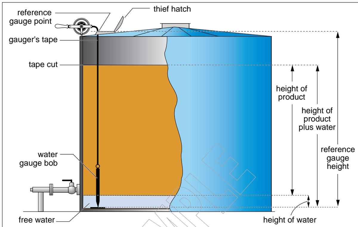
Free water gauging is relatively accurate when the density differential between the oil and water is large and when the liquid in the tank is not emulsified. If the liquid is emulsified (i.e., if the water has **not** separated from the oil), the tank contents must be sampled and the sediment and water must be measured to determine more precise oil and water volumes.
