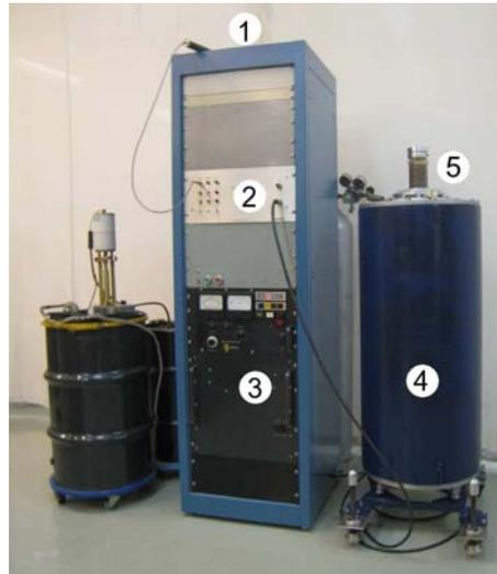
**Figure 1.** Experimental set-up. (1) Hand held 80 V trigger, (2) 50 kV trigger circuit, (3) Controller of 40 kV-40 mA DC Power Supply, (4) 30-stage inductively charged Marx Generator with the peaking capacitor, and peaking spark gap and (5) Load. This load can be either the MCG-like coil, the oscillatory circuit with the gas discharge switch assembly, BWO or the X-ray diode. DC Power Supply barrel and the charging barrel are placed on the left of the cabinet.
