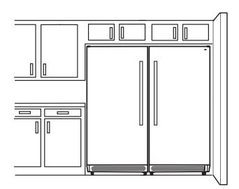
IMPORTANT: Do not install the appliances near an oven, radiator, or other heat source, nor in a location where the temperature will fall below  $40^{\circ}F$  ( $5^{\circ}C$ ).
